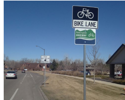
Confirmation Sign example. Credit: City of Fort Collins
