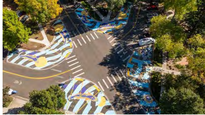
Above: An example of a painted curb extension with bollards in a residential area in Fort Collins
