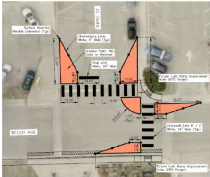
Level 2 Crossing Examples - (Top left) design for painted curb extensions near Old Town Berthoud, (Top Right) a rapid flashing pedestrian beacon on SH56 in Berthoud, (Middle Right) a raised crosswalk along the Loveland Recreation Trail, (Bottom Right) A midblock pedestrian refuge island near Rocky Mountain High School in Fort Collins
