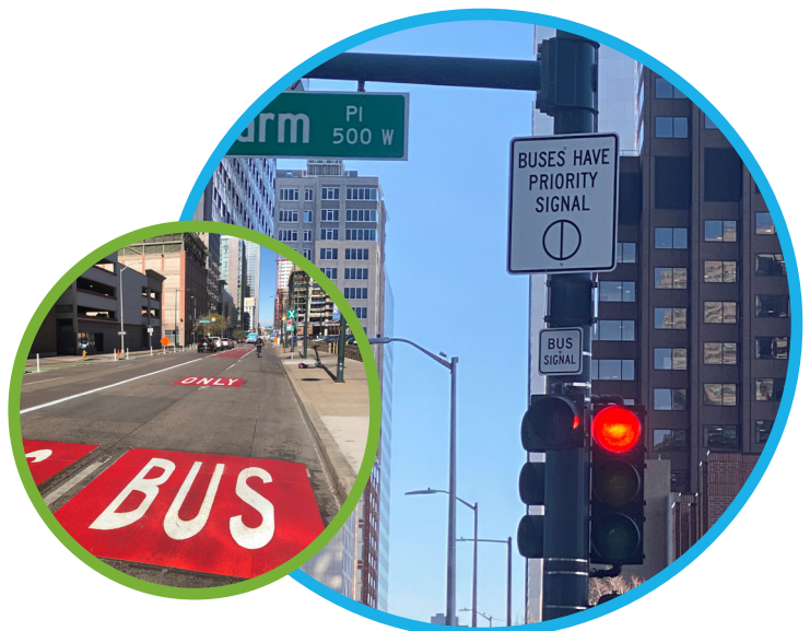
TSP systems include smart signals that can detect the location of buses and provide priority through signals.
